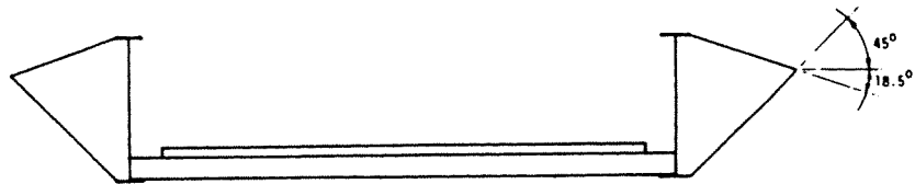
Fig. 2.b. Fairing-modified version of the Deer Isle deck section.
